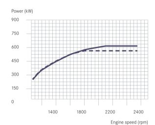
Rated Power 615 kW Rated Power 552 kW
